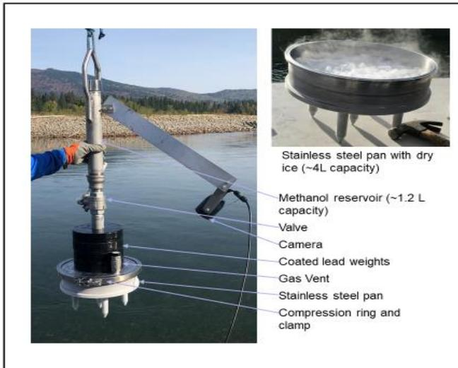
The study demonstrated that the freeze grab sampler was successful for obtaining samples in areas dominated by gravel but not for those areas where the surface sediment was dominated by cobble. CCC provided comments on the study report asking for greater specification of procedures and the use of sensor data to assess whether overlying water or groundwater was drawn into the sediment.
