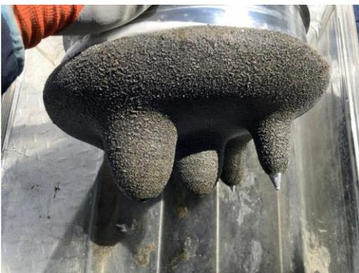
There has also been concern with prior porewater sampling techniques about the lack of ability to obtain a sufficient volume of porewater for chemical analyses without drawing in overlying water or groundwater and while avoiding oxygenation. In response to this concern, a pilot study was completed to determine if the Trident probe could be used to successfully obtain porewater samples from the variety of substrates in the UCR and across
